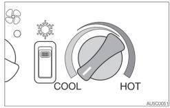
Use this dial to adjust the air temperature. COOL...... Decrease the temperature HOT...... Increase the temperature **Note:** No warm air is emitted if the temperature of the engine coolant is low.
