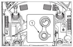
Use this socket to connect the external power supply. When using, be careful not to exceed 12V/5A.
