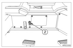
2. Press the lift arm lower button (2) to lower the lift arm.
