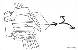
When traveling over a large step such as a cobblestone or rock (20 cm (8 in.) or deeper), climb up the step at the right angle and do not change courses on top of the step.
