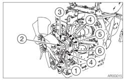
Press on the belt at the midpoint between the crank pulley (1) and alternator pulley (2) to check the tension (approx. 98 N or 22 lbf).
