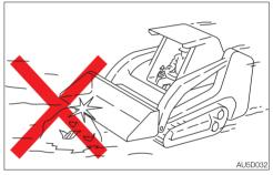
Do not allow the bucket to bump against rocks or the like. Doing so could damage the bucket and/or the cylinder.
