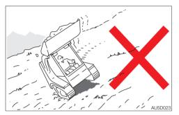
Do not perform any operation on a slope. The machine may lose its balance and tip over if the working equipment is operated on a slope.
