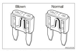
4. If a fuse is blown, replace it with a spare fuse of the same capacity.
