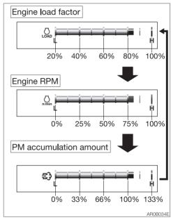
This gauge displays the load condition of the work. When the gauge is in the green range, the work load is light to medium. When the gauge is in the red range (75% or more), the work load is high. When the button (C) (Bar meter key) is pressed on a normal screen, the display changes in the following order: the engine load factor, throttle opening position and PM accumulation amount indicator.
