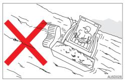
Do not cut across or go diagonally across a slope. Doing so may cause the machine to tip over or the tracks to come off and/or extremely wear.
