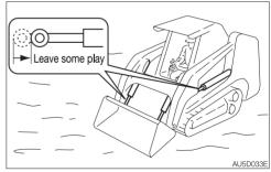
Hydraulic cylinders could be damaged due to excessive force applied, if fully extended or retracted. Allow for a safety margin when operating the cylinders.
