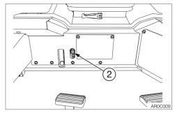
Press the lift arm lower button (2) to lower the lift arm.
