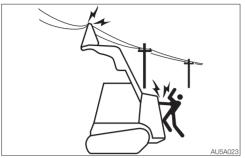
Never bring any part of the machine or loaded material to near to the high voltage cables unless all safety precautions required by the local and national authorities have been installed. If a person comes near to the machine that is discharging sparks or located near to or in contact with the power source, there is a hazard of electric shock and death.
