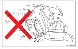
Do not attempt a spin turn or pivot turn at high speeds. Doing so may cause the machine to tip over or the tracks to come off and/or extremely wear.
