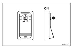
This switch controls the ON/OFF state of the high-flow function set in the auxiliary hydraulic lines.
