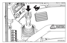
Press this button to set the travel speed to 2nd (high) speed. Press it again to return to 1st (low) speed.
