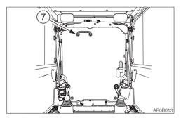
4. When the door reaches all the way down, grasp the handle (7) and firmly push the door in to engage the latch.
