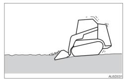
Do not dig down too deeply at a time. Doing so could damage the bucket and the lift arms.
