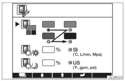
Move the cursor ▶ to the background color symbol, and then press the Enter key. The blue flashing light moves from blue gray to gray, blue and black, in this order. Move the blue flashing light to the desired color position, and then press the Enter key to confirm.
