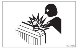
Do not remove the radiator cap or the drain plug when the cooling water is hot. Stop the engine and wait until the engine and the cooling water cool. Then, slowly loosen the radiator cap to release the internal pressure and remove it.
