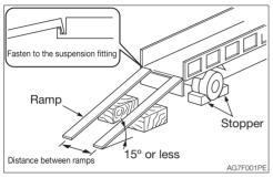
The machine may roll or tip over or fall while being loaded or unloaded. Take the following precautions:
