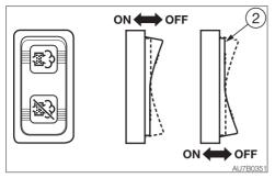
IMPORTANT: If the DPF regeneration promoting indicator lamp starts flashing and an alarm starts sounding, press the manual regeneration side (2) on the DPF manual regeneration/inhibit select switch to burn the particulate matter (PM). If the machine operation is continued without performing the manual regeneration, the engine power will decrease due to the PM excessively accumulated, and in the end, the engine will stop running.
