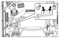
2. Open the cover and press the ⊕ side of the switch (5) to unlock the quick-hitch.
