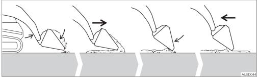
Raise the lift arms and tilt the bucket forward, then release it as the machine is driven forward. Next tilt the bucket forward and lower the front edge until it is slightly above the ground surface, then back the machine over the load that was just released.
