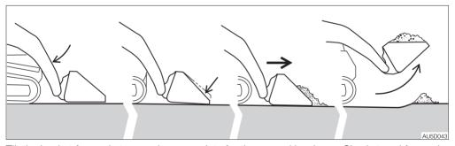
Tilt the bucket forward at an angle appropriate for the ground hardness. Slowly travel forward, dig into the ground with the cutting edge of the bucket. When the bucket is full, tilt it backward.
