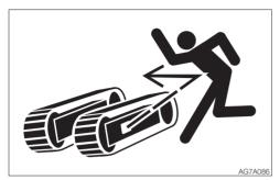
In the track adjuster, the grease has been injected under high pressure. If the tension is adjusted without following the prescribed procedure, the grease discharge valve may fly off, resulting in injury.
