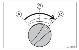
1. Turn the throttle controller and increase the engine speed.
