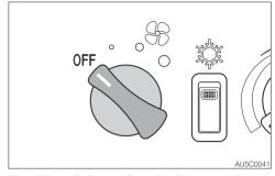
Use this switch to adjust the fan speed in three steps. Turning to the OFF position turns off the air conditioner.
