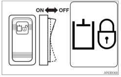
When the safety bar is lowered and the hydraulic system unlock switch is pressed, the hydraulic system lock indicator lamp goes out to indicate that the machine operation is available.
