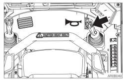
Press the button situated on the right operating lever to blow the horn.
