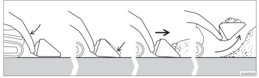
Lower the bucket to the ground and set it parallel to the ground or tilt it slightly downward. Move the machine forward, push the bucket well into the material and scoop it by rolling back the bucket.
