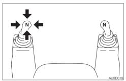
1. Set the left control lever slowly to the neutral position. The machine stops. Braking is automatically applied by the hydrostatic drive system when the left control lever is returned to the neutral position. Full braking is achieved when the safety bar is raised.
