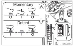
Select the operation mode for the auxiliary hydraulic button (A) by operating the detent mode switch (D).
