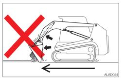
Do not fully extend the bucket cylinders, push the bucket into the ground and move the machine to use the traveling force for digging. Doing so could damage the bucket cylinders.
