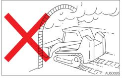
Do not use this machine in areas where there is danger of explosion from volatile gases. Also avoid using the machine where the exhaust gases could come in contact with flammable items.
