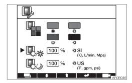
The brightness of the LCD is set to between 20 and 100%.
