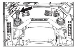
Use this lever to move forward and in reverse and to change directions.
