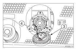
4. Remove the DEF/AdBlue® tank cap (3).
