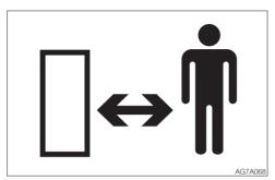
Do not allow unauthorized personnel in the work area while working. Be careful when grinding, welding or using a hammer. You could be injured by flying debris from the machine.
