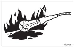
To prevent an ignition or explosion, use explosion-proof lights when inspecting fuel, oil, coolant or battery fluid. Otherwise, explosion could result causing serious injury or death.
