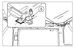
6. Get in the cab and insert the lock pin (5) into the pin hole on the cab to lock it.
