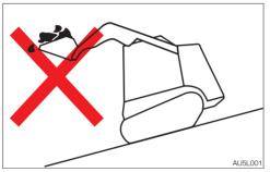
Traveling down the slopes with the attachment raised
