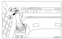
2. Press the auxiliary hydraulic button (A) or slide the slider switch to the left side (A).
