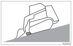
If you must park on a slope or incline, park the machine securely and block the movement of the machine.
