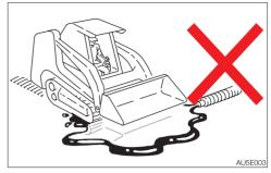
Do not let fuel, oil, salt or chemical solvents get on the tracks. These substances may corrode the bonding of the steel cores on the tracks, resulting in rust or peeling. If any of these substances gets on the tracks, immediately clean it off with water.
