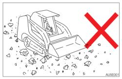
Traveling and slewing on crushed rock, extremely rough hard rock, steel beams, scrap iron, or near the edges of steel plates will cause damage to the rubber tracks.
