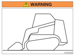
• Park the machine on a flat, rigid and safe ground. Set the parking brake.
