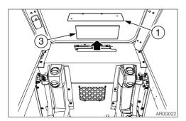
1. Lift the filter (3) and remove it.
