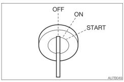
IMPORTANT: Do not repeatedly switch the key from OFF to ON and ON to OFF over a short period. Doing so will cause engine breakdown.
