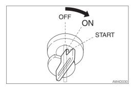
5. Insert the key into the ignition switch, turn it to the ON position, and then perform the following inspections:
