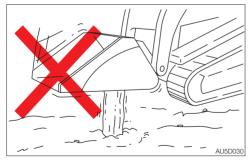
Do not use the downward force of the bucket to drive piles.
