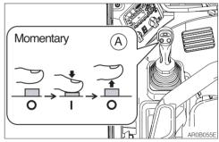
These switches stay on while the buttons are pressed; they turn off when the buttons are released (momentary mode).
