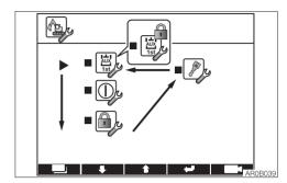
The settings made to the machine can be changed. Move the cursor ▶ with the Up (↑) or Down (↓) key to go to the desired item to be set, and then press the Enter key to confirm.
