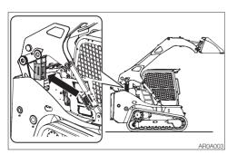
Never leave the machine with the engine running or the lift arms raised. If the lift arms are left in a raised position, prevent them from falling by engaging the lift arm stopper.
