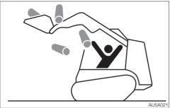
Unstable loads such as round items, cylindrical items, and stacked plates may fall from the bucket. When handling unstable load, do not raise the bucket too high or tilt it backward too far.
