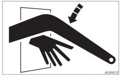
It is dangerous to operate the machine while putting your arms, feet or legs out of the operator's compartment. Never do it.
