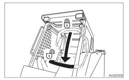
Lower the safety bar completely down to the unlock position, and then press the hydraulic system unlock switch to release the hydraulic system lock.
