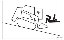
Opening the door while traveling on slopes is dangerous, as the force required to open and close the door changes abruptly. Always keep the door closed when traveling on slopes.
