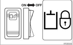
2. Lower the safety bar completely down to the unlock position, and then press the hydraulic system unlock switch to release the hydraulic system lock.
