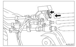
Note: This device works as a safety device to prevent accidental activation of the attachment or hydraulic quick-hitch installed. When the attachment hoses are connected to the quick-coupler, the plate is pushed to turn on the switch, which prevents the hydraulic quick-hitch from being activated even when the lock/unlock switch on the hydraulic quick-hitch is pressed. When the hydraulic quick-hitch needs to be activated, disconnect all hoses from the quick-coupler.
