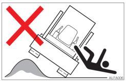
Traveling over obstacles (rocks, stumps, etc.) may put a great load on the machine body and may cause damage to it. Avoid crossing over obstacles whenever possible. If you must do so, keep the bucket near the ground, travel at a low speed, and go over the obstacle at the center of the track.
