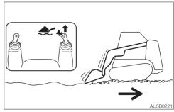
➤ To float the lift arms: Tilt the right control lever forward a little and depress the float button. Refer to "Float button" on page 2-37.
