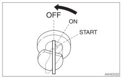
3. Turn the ignition key to the OFF position to stop the engine.
