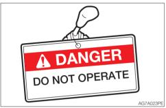
Display a "DO NOT OPERATE" alert sign on easy-to-see locations such as on the ignition switch or on control levers.
