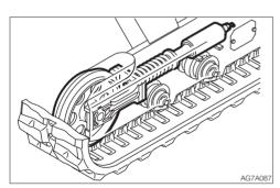
There is a very strong spring contained in the track adjuster. If the track adjuster is accidentally disassembled, the spring can pop out, resulting in serious injury Never disassemble the track adjuster.
