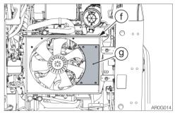
5. Remove the plate (g) from the fan shroud
