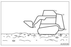
On uneven ground, maintain the low speed and avoid starting, stopping or changing directions abruptly.
