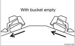
When traveling on slopes of 15 degrees or more, position the heavier end of the machine (front or back, whichever is heavier) pointing up the slope. Also, be careful not to tip over or slide.
