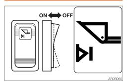
The self-leveling function is enabled or disabled with this switch.
