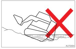
If the rear of the machine is submerged in water as shown in the figure above, it causes the radiator fan to turn in water, resulting in damage to the fan. The rear of the machine must not be submerged.
