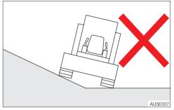
Avoid traveling by setting one track on a slope or projecting portion and the other track on a flat surface (with the machine at a tilt of 10° or more). Travel with both tracks set on flat surfaces.
