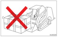
Do not use this machine beyond the specifications or overfill the bucket.
