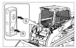
This switch is used to shutdown the engine if it fails to stop, due to machine failure or breakage, when the ignition switch is set to the OFF position.
