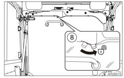
If the release lever (6) does not work, move the emergency unlock lever (8) to the left to release the latch.
