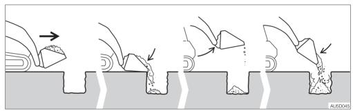
With the bucket lowered, drive near the hole and tilt the front edge of the bucket downward as soon as it passes over the near side of the hole. Raise the bucket and empty the load only when necessary.
