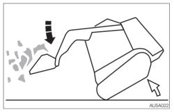
Sudden lowering or stopping of the working equipment could cause the machine to react and tip over. Operate the working equipment carefully, especially when the bucket is loaded.
