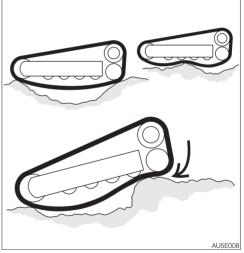
• Do not change directions when the tracks are slack as shown in the figure.
