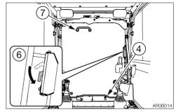
1. Pull the release lever (6) to release the latch.
