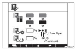
Switch between SI unit and US units. Move the blue flashing light to the desired unit position, and then press the Enter key to confirm.
