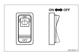
ON .....Pressing the ON side of the switch causes the washer to spray washer fluid. To stop spraying, release the switch.
