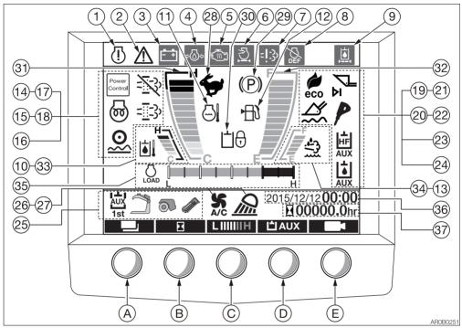
For explanation purposes, all lamps on this page are in the lit condition. This screen image is quite different from that of the real operation. In the actual operation, if a warning is given or any function is selected, the corresponding symbol appears enlarged at the center of the display for approx. one second.
