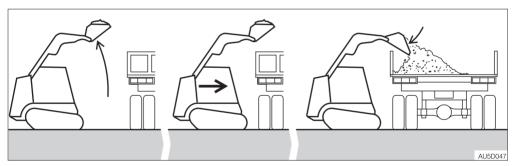
Move the machine, stop close to the truck, and then raise the bucket until its lower edge is well above the truck bed. Slowly move the machine forward and stop at the position where the bucket is to dump. Tilt the bucket forward to release the material in the bucket into the truck bed. When the truck bed is filled to half capacity, use the bucket to spread the load evenly.
