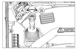
Proportional control allows for slow-to-fast movement of auxiliary functions. Example: If you move the slider switch half way, the auxiliary function will move at approximately one-half speed.
