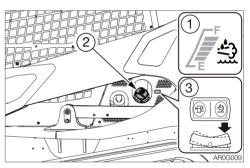
Use the DEF/AdBlue® level indicator to check the amount of DEF/AdBlue® solution remaining.
