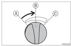
1. Turn the throttle controller to the middle position, then run the engine at medium speed for about 5 minutes with no load.
