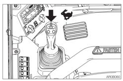
Press the travel speed button on the left control lever to switch to 2nd (high) speed, and press it again to return to 1st (low) speed.
