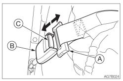
1. Grasp the tongue plate (A) and press the button (C) on the buckle (B).
