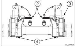
8. Push both lock levers (2) until they are horizontal to engage the latch.
