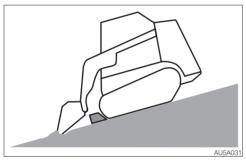
If you must park on a slope or incline, park the machine securely and block the movement of the machine.
