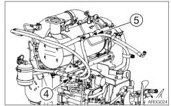
5. Check the temperature of the compressor's high pressure pipe (4) and low pressure pipe (5).
