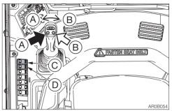
Press auxiliary hydraulic buttons (A) or (B) to control the flow of the oil in the auxiliary hydraulic circuit.
