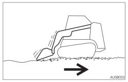
While in the float mode, the bucket moves up and down in response to the "bumps and dips" on the ground surface.
