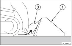
Slowly move the machine forward and raise the lift arms. Engage the wedgeshaped top edge of the quick-hitch (3) onto the bucket (1) upper part (quick-hitch mount).
