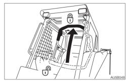
Raise the safety bar to the locked position, and then check that the control levers are locked.
