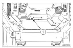
1 Remove the rubber (1) from the top of the button.
