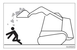
The load spilling or the bucket dropping may occur while the bucket is over the heads of people.
