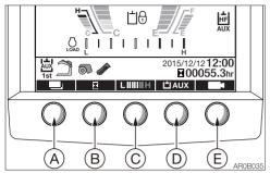
**Note:** Do not press the symbol keys on the display. The LCD could be damaged if the symbol keys are pressed hard. For actual operation, press the push button keys located at the bottom of the screen.
