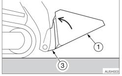
5. Tilt the quick-hitch (3) backward while lifting the bucket (1) off the ground. The quick-hitch (3) will slide into position.
