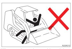
When operating any lever, pedal or switch, always do it while sitting in the operator's
