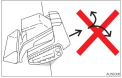
When climbing in reverse, do not change directions at the point where the slope starts.
