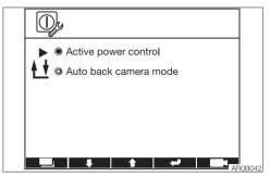
The active power control and the auto rear view camera mode can be set to ON or OFF. To return to the machine setting screen, press the Menu key.
