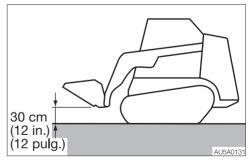
3. Roll back the bucket all the way, and then lift it to 30 cm (12 in.) above the ground.
