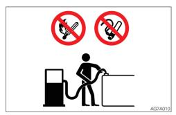
Keep flames away from fuel, oil, grease and antifreeze. Fuel is particularly flammable and dangerous.
