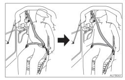
IMPORTANT: To prevent the belt from falling off the shoulder and contacting your arm or neck, wear the belt in such a way that it is rested over the center of your shoulder.
