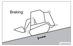
When descending slopes, the brakes are applied automatically once the control levers are returned to the neutral position.
