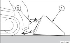
3. Tilt the quick-hitch (3) forward to disconnect its upper edge from the bucket (1) upper part (quick-hitch mount).
