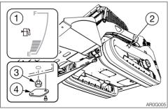
1. Check the fuel level using the fuel gauge (1).
