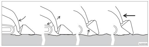
Lower the bucket to the ground before setting the lift arms to the float mode. Tilt the bucket forward to stand it on its cutting edge, and then level the loose ground while driving in reverse.
