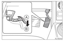
This controls the engine speed.
