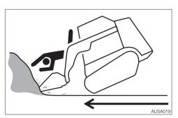
Driving at high speed into the materials you are handling can lead to your body striking the machine or being thrown from the machine. Before working the material, check the conditions of the area and work at low speeds.
