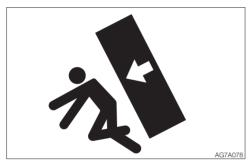
When it is necessary to temporally place a heavy object, bucket or an attachment on the ground during removal or installation, be sure to place it in a stable position. Keep off unauthorized persons from the storage place for such object.
