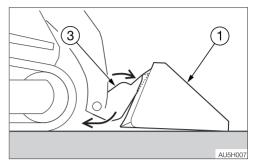
Tilt the quick-hitch forward to disconnect its upper edge from the bucket (1) upper part (quick-hitch mount).
