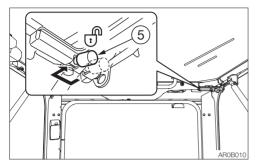
1. Remove the lock pin (5) from the pin hole on the cab to release the door lock.
