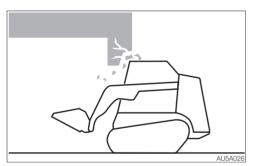
Check the height limit and width limit of tunnels and bridges beforehand to avoid the machine from contact with the ceiling or walls. If contacted, it could result in a serious accident.
