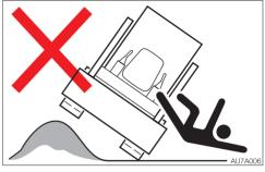
Avoid crossing over obstacles whenever possible. If you must do so, keep the bucket close to the ground level and travel slowly. Never cross obstacles which will tilt the machine to an angle of 10° or greater.
