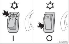
Use this switch to turn on or off the air conditioner. When this switch is pressed while the engine is running and the fan switch is on, the air conditioner turns on. Press this switch again or turn the fan switch off to turn off the air conditioner.
