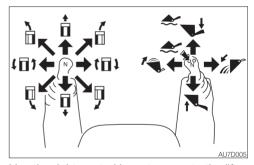
Use the right control lever to operate the lift arms and bucket.
