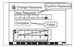
The password can be changed. Use the Up (↑) or Down (↓) key to move the cursor ▶ to the password field, and then press the Enter key to enter a 4-digit number password. Once the password is entered, the display of "New Password" is change to "Confirm Password".
