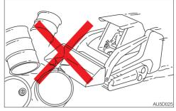
Travel at a speed appropriate for the operating conditions. Travel at low speeds with care in the places where the field of view is obstructed or there are hazardous objects nearby.
