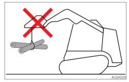
The machine is NOT specifically designed for lifting loads and has no safety devices for crane operation.
