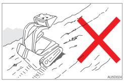
Do not travel or turn with the bucket raised. Keep the bucket as low as possible during traveling.
