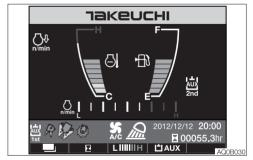
Turn on the light switch on any screen to decrease the display brightness and to enter the "evening mode".
