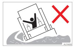
Driving on the soft ground could cause the machine to tilt under its own weight, resulting in a machine tipping over or sinking into the ground.
