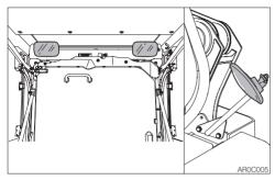
Adjust the rear view mirrors to have a better rear view.
